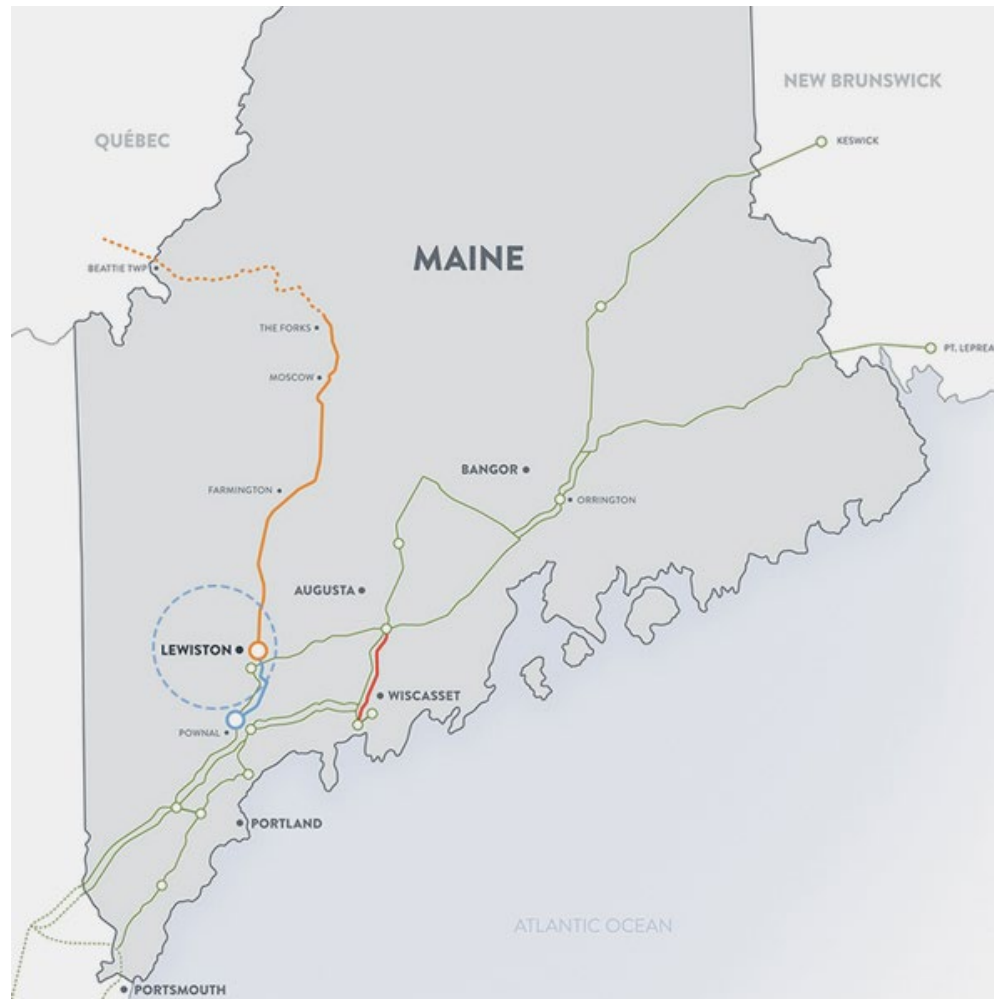
Although most of the 145-mile New England Clean Energy Connect transmission line would follow existing utility paths (solid orange line), it would require removing trees for 53 miles through western Maine (dotted orange line). | Avangrid
