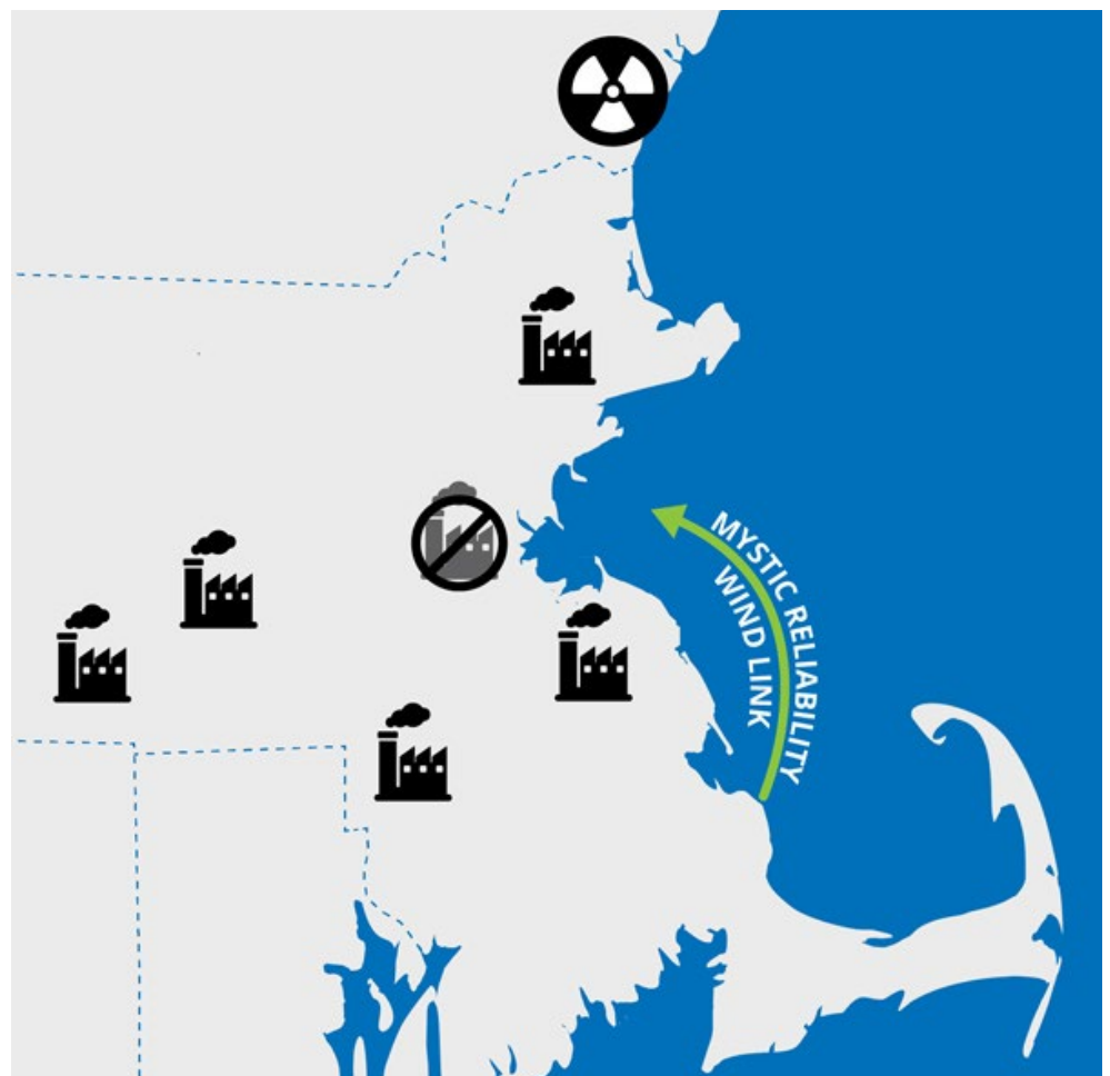
Anbaric’s proposed Mystic Reliability Wind Link would bury transmission cables underground and under the seabed from Plymouth, Mass., to Everett, Mass., site of Exelon’s Mystic Generating Station. | Anbaric Development Partners
