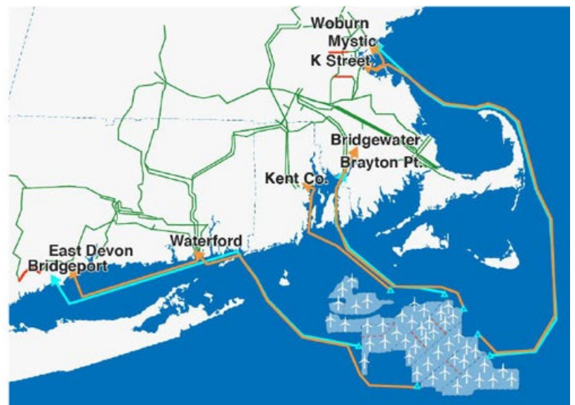
The Brattle Group compared two different scenarios: one in which each offshore wind project interconnecting to the grid uses its own individual line (left), and another in which a shared, open-access offshore grid is planned. | The Brattle Group
