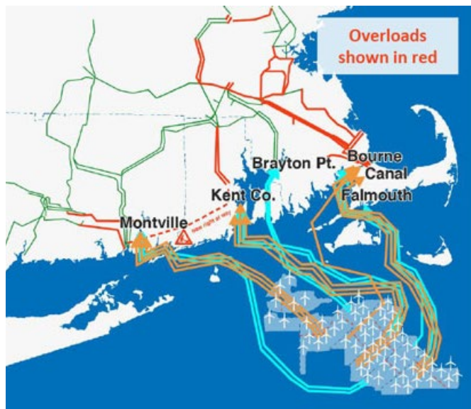
The Brattle Group compared two different scenarios: one in which each offshore wind project interconnecting to the grid uses its own individual line (left), and another in which a shared, open-access offshore grid is planned. | The Brattle Group
