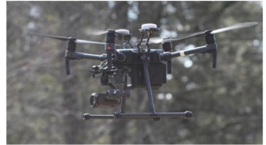
High-definition cameras on drones allow Eversource Energy line inspectors to see possible damage from all angles and take better photos. | Eversource
