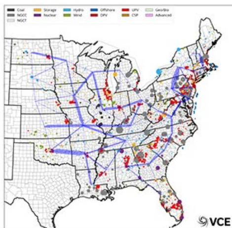
Transmission expansion (2030) under a strong carbon/high solar deployment (left) and strong carbon/high wind deployment | Americans for a Clean Energy Grid
