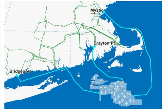
Generator lead line vs. planned mesh network for New York | The Brattle Group
