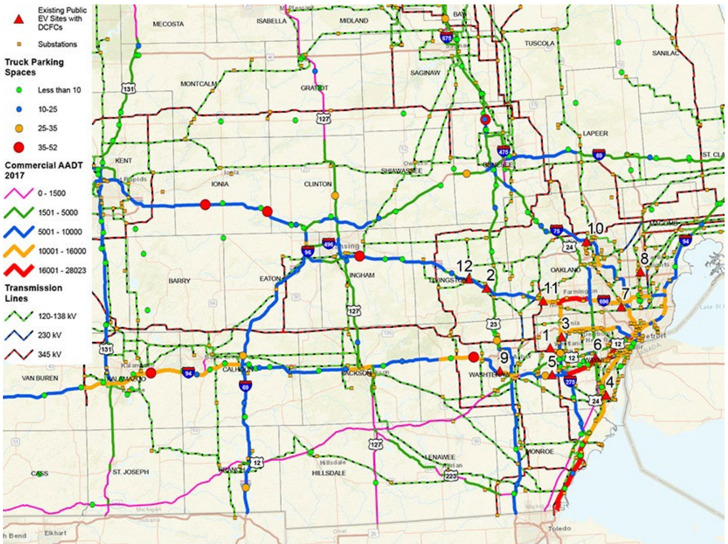
This map overlays electric transmission with average annual daily traffic (AADT) and locations of truck stops and existing DC fast charging spots in Michigan. | HDR Inc.
