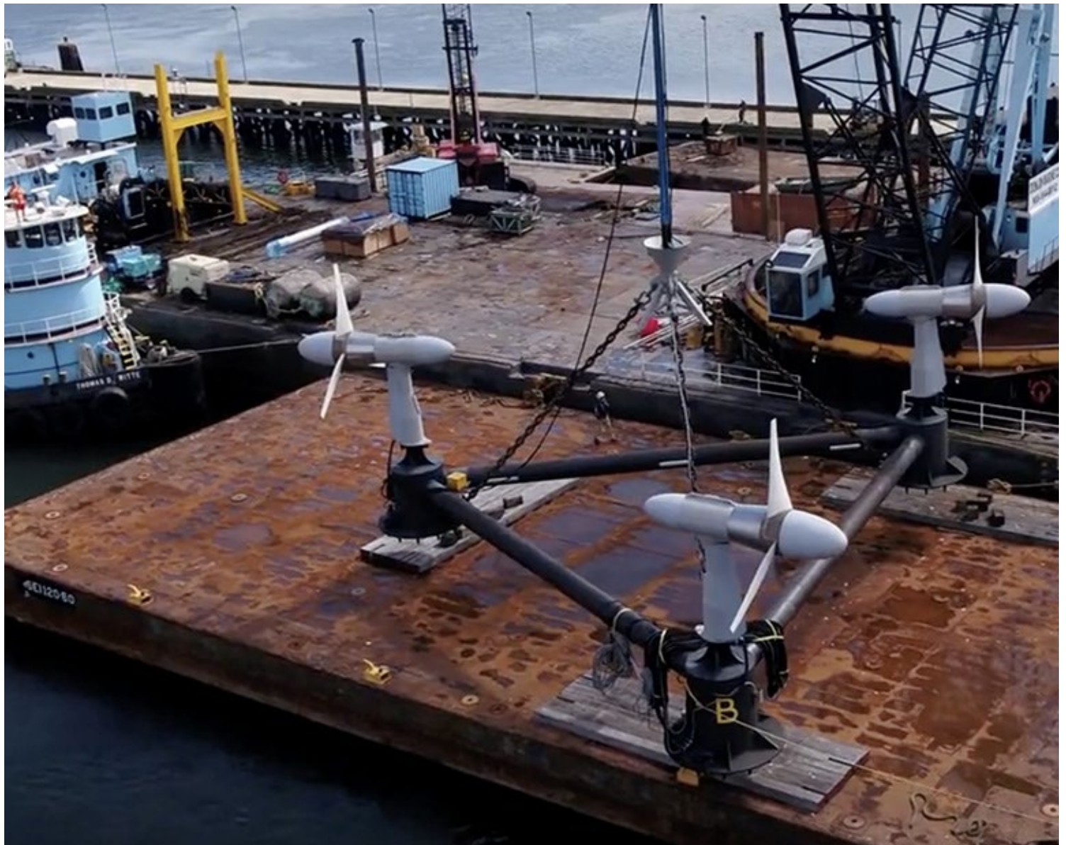
Roosevelt Island Tidal Array: Verdant Power's project of three tidal power turbines in the East River is an example of new renewable energy resources coming onto the grid. | Verdant Power
