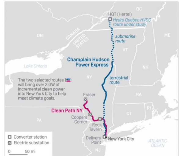
Transmission sensitivity assumptions in the market impacts study include over 2.5 GW on two high voltage direct current (HVDC) transmission lines into New York City. | Analysis Group
