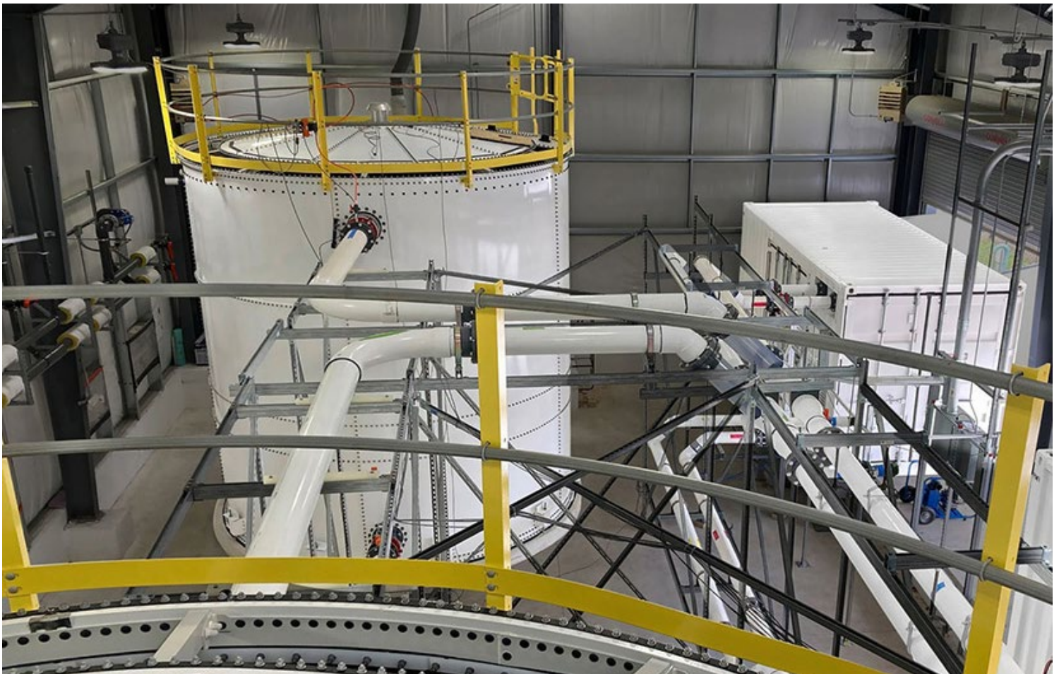
Lockheed Martin is testing the first commercial model of its GridStar flow battery at its research facility in Andover, Mass. | Lockheed Martin
