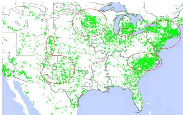
Operating and planned wind and solar projects as of 2020. The ovals represent areas of high wind and solar siting along interregional interfaces, which could potentially benefit from greater interregional transfer capacity. | ABB Hitachi
