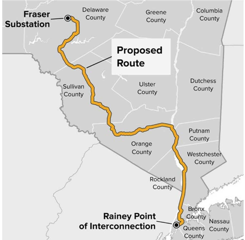
The CPNY project includes a new 174-mile, 1,300 MW HVDC transmission line to the Rainey station in Queens, while the CHPE would run 339 miles from the Canada-US border to the Astoria substation in Queens. | NYSERDA
