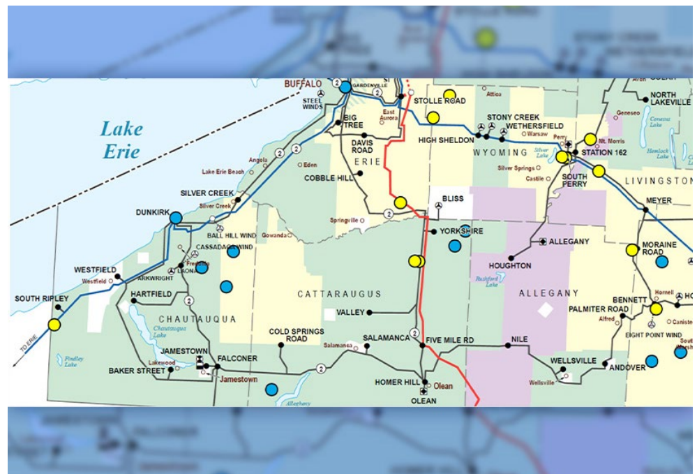
Niagara Mohawk map showing its southwest territory and 18 circuits, of which 13 circuits are 100 years old or older, contributing to "bottling" of new renewable generation. | National Grid
