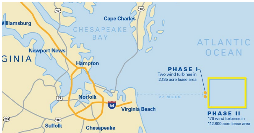
Dominion Energy's 2.6-GW Coastal Virginia Offshore Wind would be located in a 112,800-acre lease area just east of its two-turbine pilot project, 27 miles off the coast of Virginia Beach. | Dominion Energy
