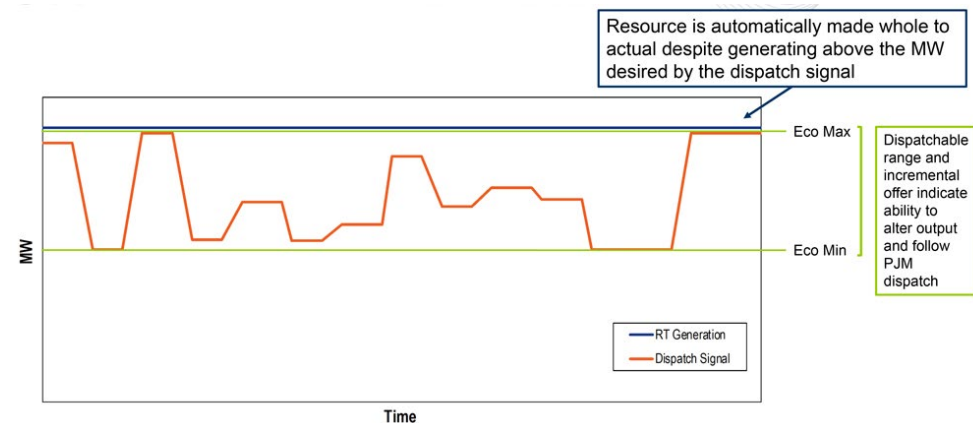
The distance between the orange (dispatch) line and blue (actual operation) line represents excess MWs for which the combustion turbine can receive make-whole payments under current PJM rules. | PJM
