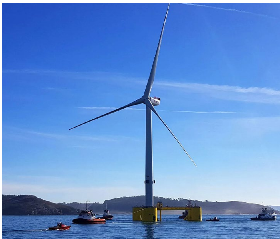
Floating wind turbines off the California coast could surpass current installations in Europe, measuring up to 900 feet tall and generating 15 GW each. | Principal Power
