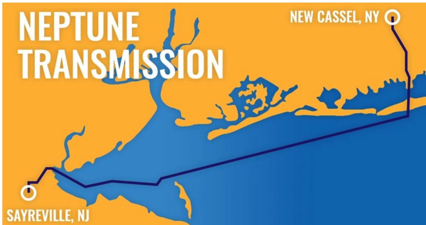
Neptune operates a 660-MW 65-mile undersea and underground HVDC line from Sayreville, N.J. to Nassau County, Long Island under a long-term agreement with LIPA. | Neptune Regional Transmission System
