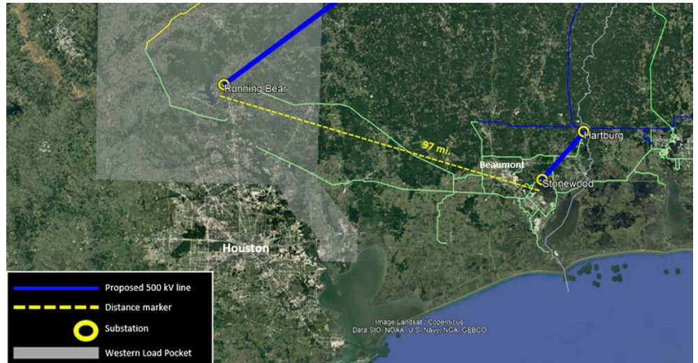
The proposed $1.1 billion, 500-kV baseline reliability project submitted by Entergy Texas under MISO's 2023 transmission planning cycle | Entergy Texas and Google
