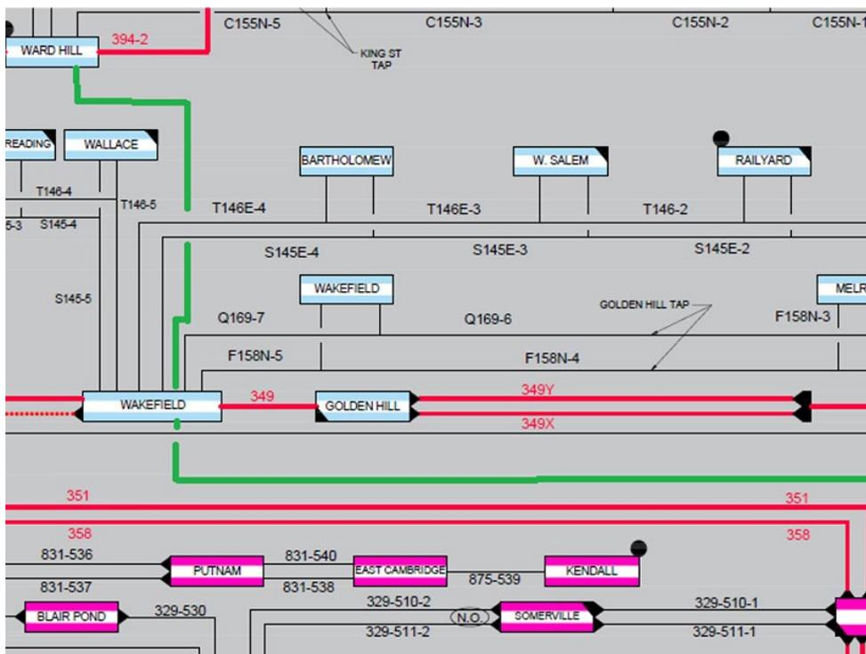
One potential transmission solution to accommodate high flows into the Boston area under both summer and winter peak conditions is the installation of a 345-kV AC line from Ward Hill to Wakefield Junction to Mystic (shown in green). | ISO-NE
